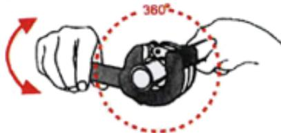
Pull knob out, down and release in a single action to start cutting procedure.
