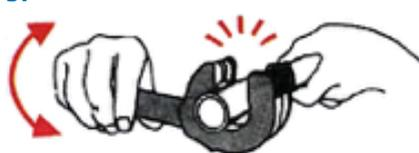
Tighten tool around the tube when needed. Repeat each action until tube is cut.
