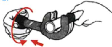
Rotate clockwise to tighten jaw grip.
