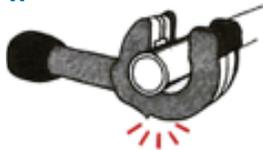
Place tube securely between cutter jaws.
